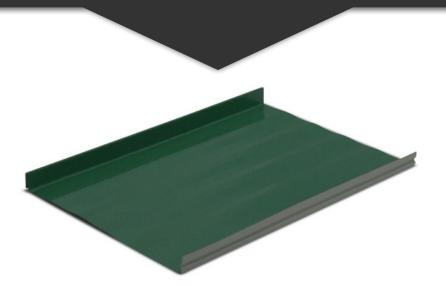
Endura Seam offers an unmistakable combination of innovation and strength, with thin-seam 1.5" high ribs at 15.625" apart. UL90 hidden Clip-Tech side laps allow unlimited expansion and contraction and seal out the weather.
