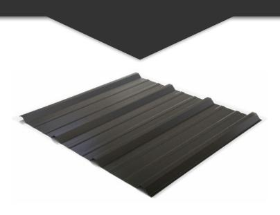
R-Panel/PBR-Panel is a low slope metal roof and wall panel with 1.25" high ribs at 12" apart. R-Panel/PBR-Panel installs quickly and cost efficiently on slopes as low as 1:12 - it's our most popular panel chosen for commercial and agricultural use.
