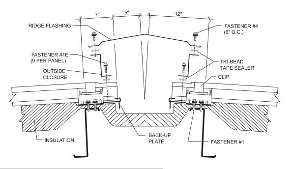
Install the ridge flashing starting and ending 2Z\x" outside the steel line. Fasten the ridge flashing to the outside closures with Fastener #4. Install a fastener 1Z\x" from panel seam on both sides of panel. Install additional fasteners directly above minor ribs of panel. Four fasteners are required at each panel. Leave 6" unfastened on each end to allow for the rake trim to be installed later. DO NOT FASTEN THROUGH THE LOCK OF THE STANDING SEAM.
