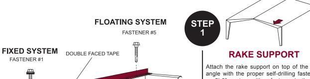
Attach the rake support on top of the rake angle with the proper self-drilling fasteners on 2'-0" centers with a fastener in the first and last prepunched slot. The vertical leg is to be installed square with the eave. Center fasteners in slots.
