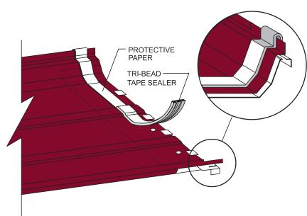
Install Tri-Bead tape sealer over prepunched holes. Be sure to place the tape sealer over the male leg. DO NOT REMOVE THE PROTECTIVE PAPER AT THIS TIME, EXCEPT AT THE MALE LEG.
