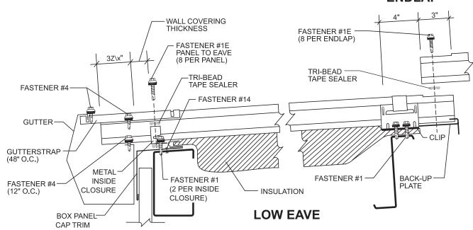
NOTE: THE ABOVE GUTTER SHOULD NOT BE USED IN AREAS THAT EXPERIENCE SNOW LOADS OF 10 PSF OR HIGHER. SEE PAGE 59 FOR THE GUTTER DETAIL FOR THESE AREAS.
