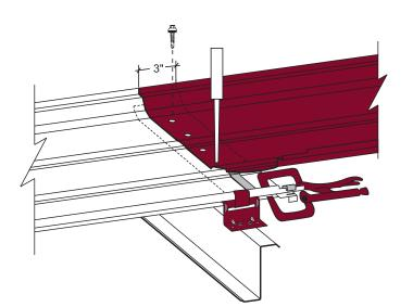
Remove awl and insert in the middle hole nearest the male leg. Install Fastener #1E in the hole by the female leg.
