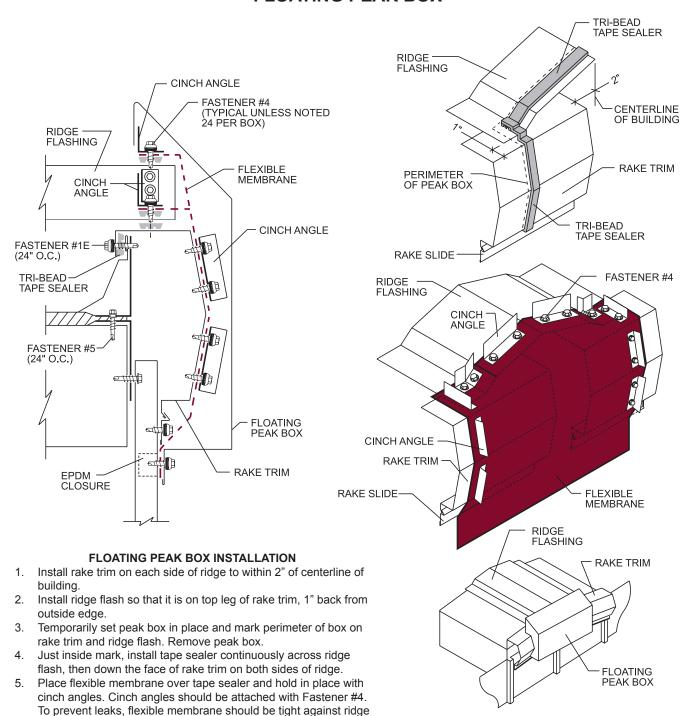
flash and rake trim with no wrinkles at the sealed edges.6. Hook top of peak box over cinch angles installed on top of ridge flash and attach bottom of peak box to endwall with Fastener #4.
